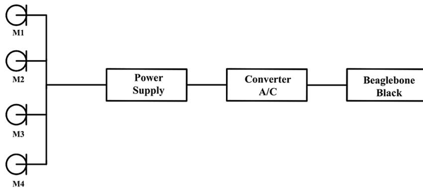
Figure 3. Elements of the assembled measuring track
