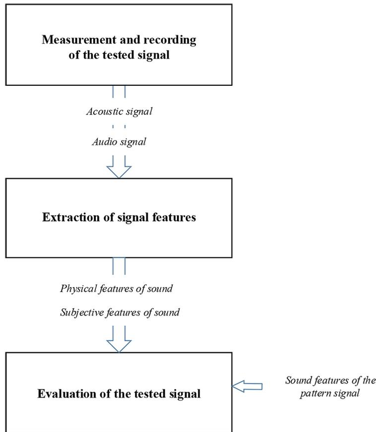
**Figure 1.** Scheme of processing the sound features of the tested signal for the needs of their assessment
