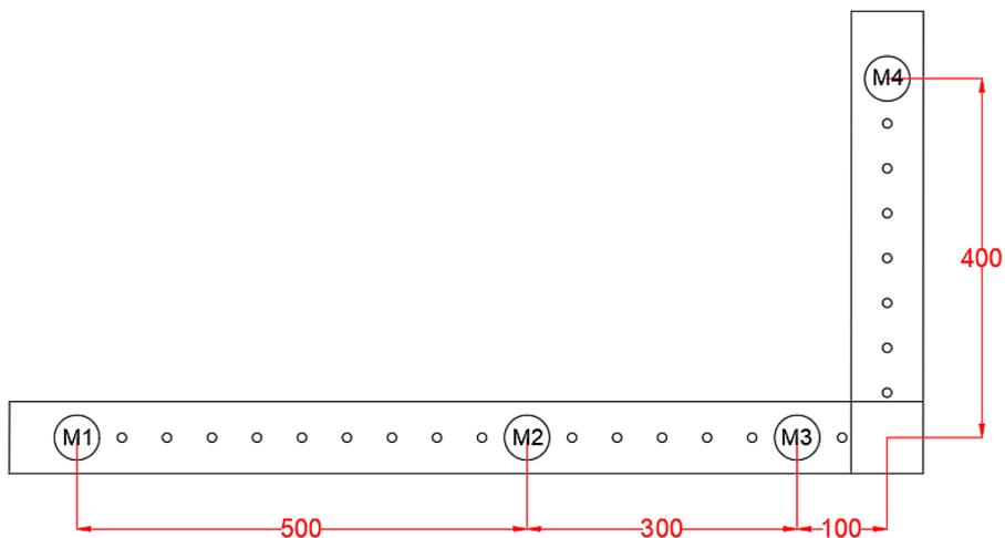
Figure 4. Arrangement of mounting strips with the adopted location of microphones
